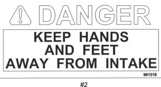
Replace safety signs immediately should they become damaged, torn or illegible. Obtain replacements from your authorized dealer using the part numbers shown.
